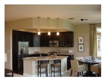
See the sprinkler head? Most sprinkler heads in homes are concealed giving them a very low profile. A smoke detector has a larger profile than a fire sprinkler head.
